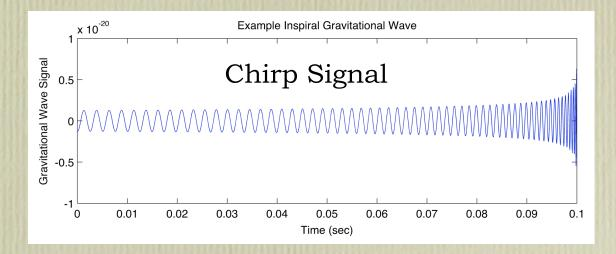
The shrinking will make GWs increase in freq. and amp. This is called a chirp signal.
