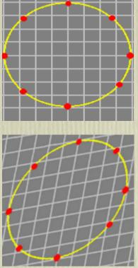
• the circular polarization  $h_{+}^{\text{TT}} = h_{\times}^{\text{TT}} \neq 0$
